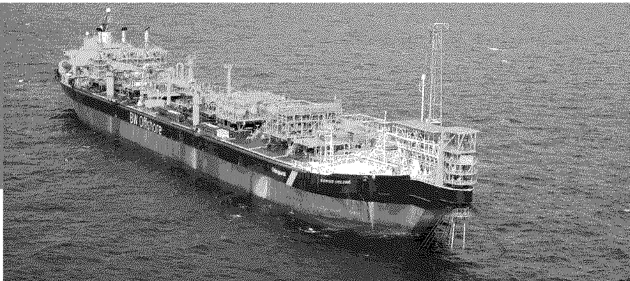
On the Berge Helene more than 6,000 tonnes of processed steel went in to strengthening the ship as part of turning it from a ship into a floating production, storage and offloading vessel (FPSO).
