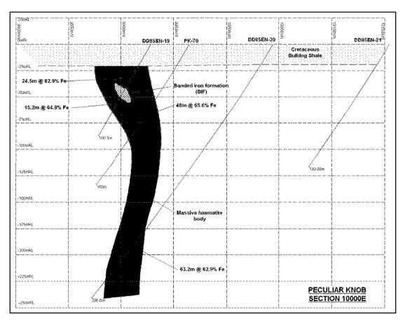
WPG notes that the continuity of mineralisation shown in the diagram above is good, the iron grades are high, and that the deposit extends to a depth of more than 250 metres on this section.
