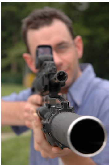
Above: the 3GL mounted on a SAR 21 Bullpup Assault rifle using a picatinny rail. Note the ergonomics of the trigger assembly in conjunction with the rifle itself.
