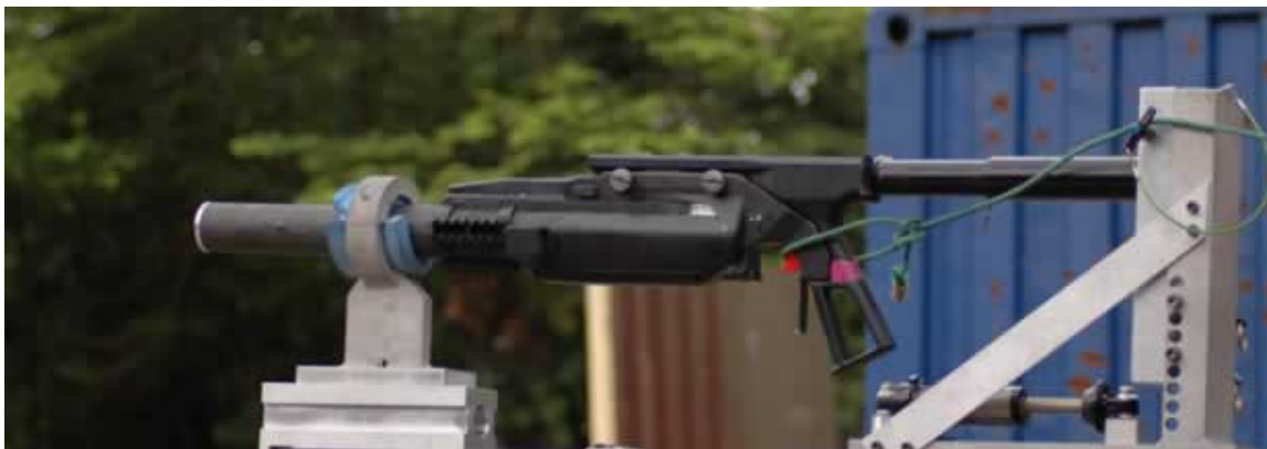
Above: 3GL mounted on a standalone shoulder stock, on a rig for test firing. Note the rope used to activate the trigger – proving the weapon is fully integrated for the firing tests.
