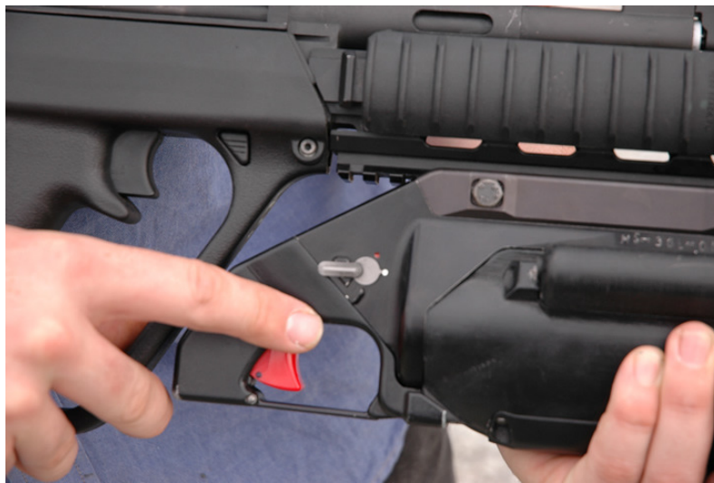
Above: the 3GL mounted on a SAR 21 Bullpup Assault rifle using a picatinny rail. Note the ergonomics of the trigger assembly in conjunction with the rifle itself.
