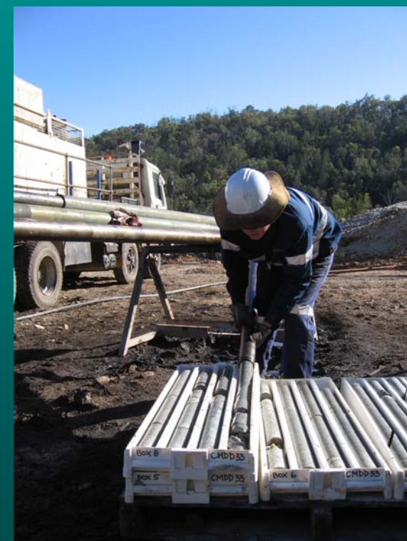
UNLOADING CORE FROM DRILL STEM
