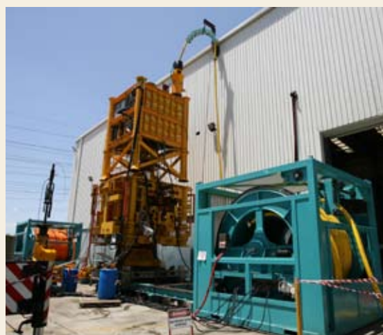
The new well intervention equipment undergoing final integration testing in Perth with a Vincent subsea tree (wellhead) in the centre. Installation of the Vincent subsea tree in 2008, will be the first time this type of equipment has been used in Australia.
