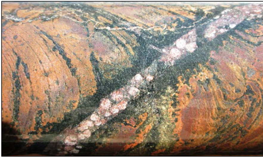
Photo 5: Multiple alteration and vein phases in contorted sediments with magnetite replacing fractured bedding (Approx. downhole depth 956m).
