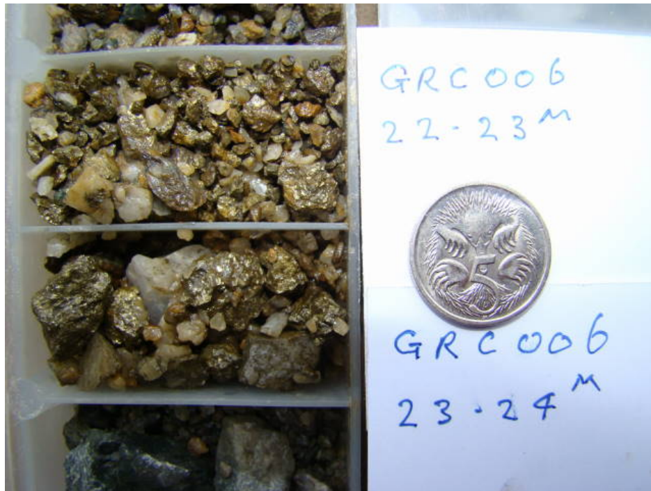
Plate 1: Chip trays showing sulphide-rich nature of samples within hole GRC006. The 1m sample between 22-23m assayed 86.4 g/t Au and the interval 23-24 assayed 59.6 g/t Au
