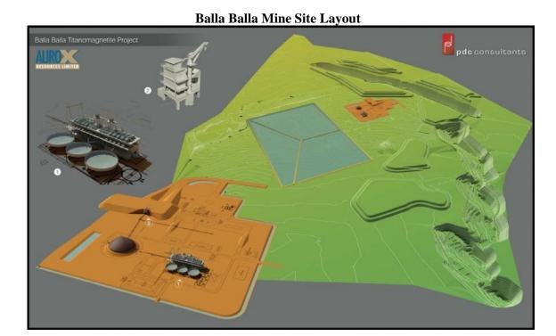
The footprints at the plant and the port sites have been designed for the increased throughput rates, with nominated areas for the extra magnetic separation units, tailings thickener and dewatering filters. The 3D modelling and general arrangement drawings depict the layouts after the expansion to 10 Mtpa production.
