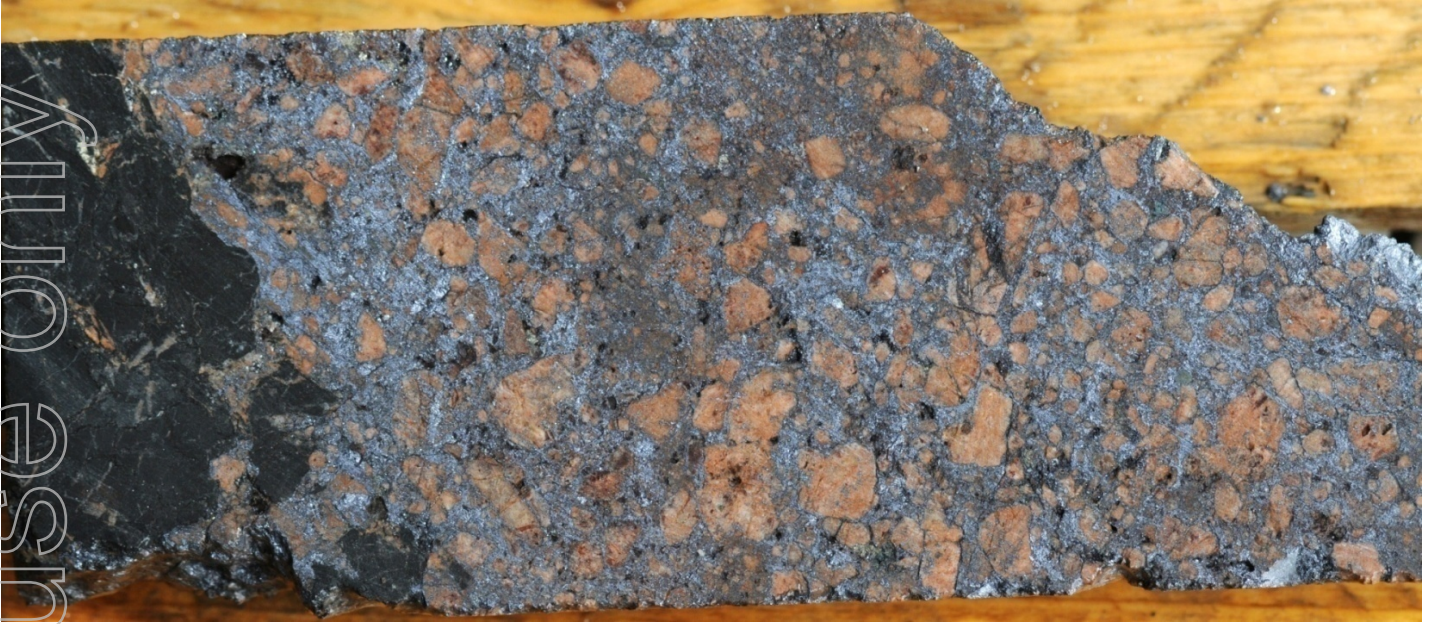
Figure 10: MDQ0147 – 238.4 – Interval from 238-239m, 12.4% Mo, 305g/t Re, 0.6% Cu, 0.16g/t Au, 83g/t Ag
