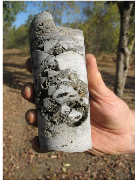
Plate 2: Sphalerite in replacement breccia, BDD002
