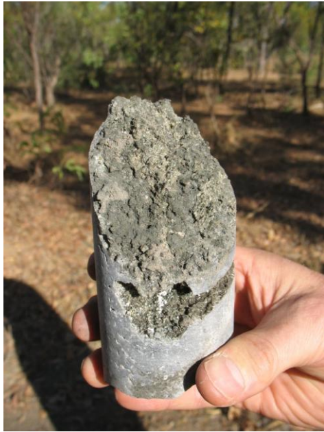
Plate 1: Sphalerite on vug and fracture plane, BDD001
