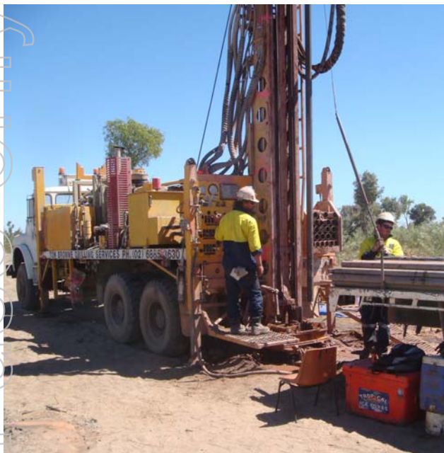
Diamond core drilling at Calvert Hills
