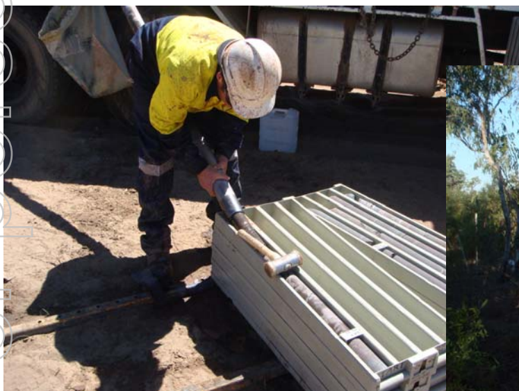
Retrieving core samples from the drill string
