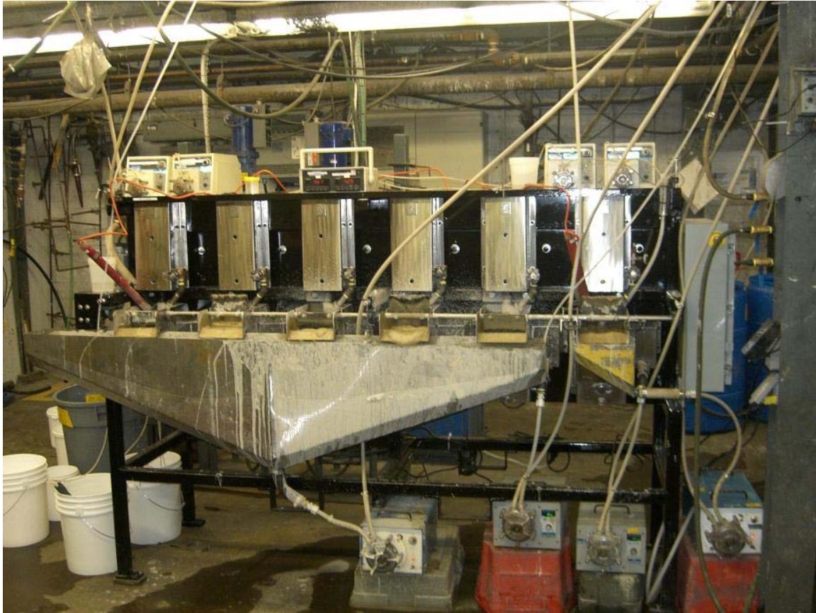
Figure 1. Mini flotation concentrate production plant in operation at SGS Lakefield, Canada.
