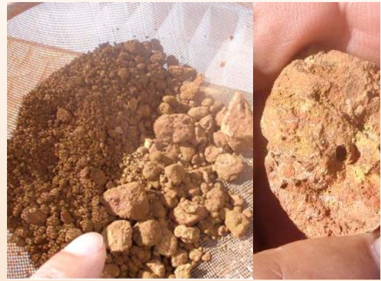
Drillhole 46: Sieved sample from 1 – 2m depth 47% Al 2 O 3 1.7% SiO 2 21% Fe 2 O 3 26% LOI
