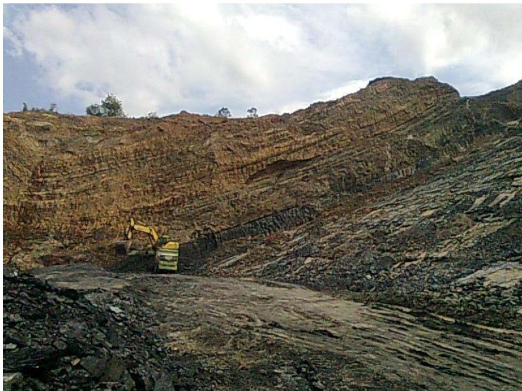
Mining on adjacent block exposing the BBPK Coal Seam (Note Outcropping seam on top right corner of Photograph)
