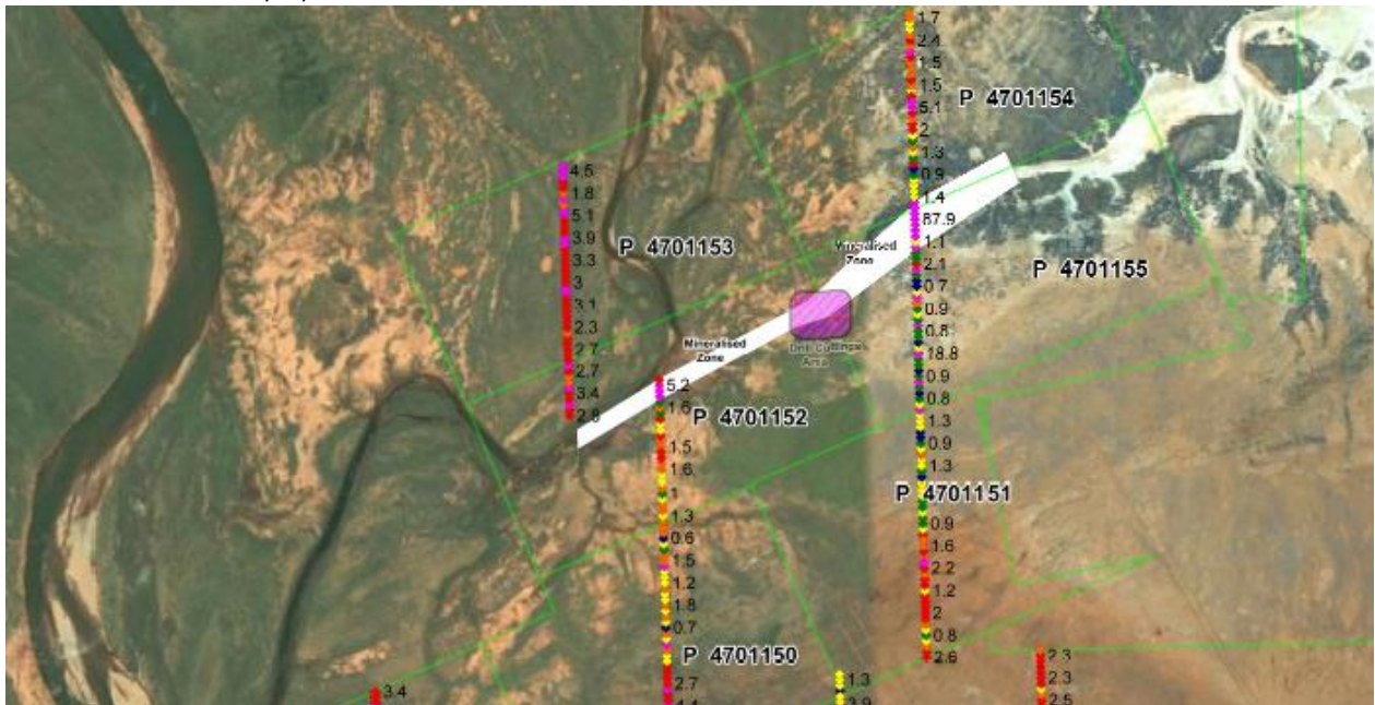
Figure 2 Biogeochemical Results: Zone of anomalism in white, area of historic drilling in pink. Biogeochemical Nickel assays coloured by percentile, with pink representing the top 5% (highest grade).
