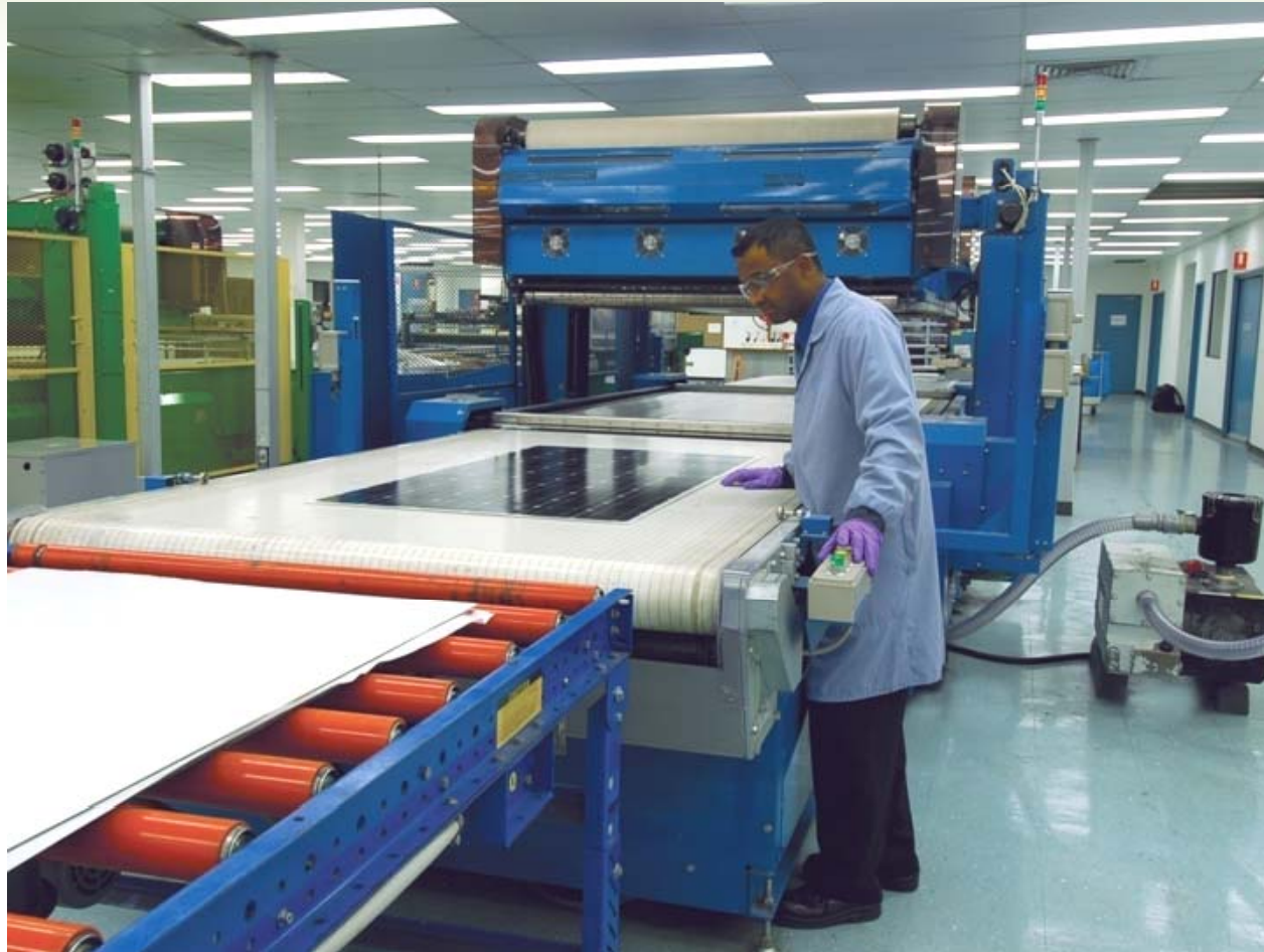
Solar Module Process Line (Laminator)
