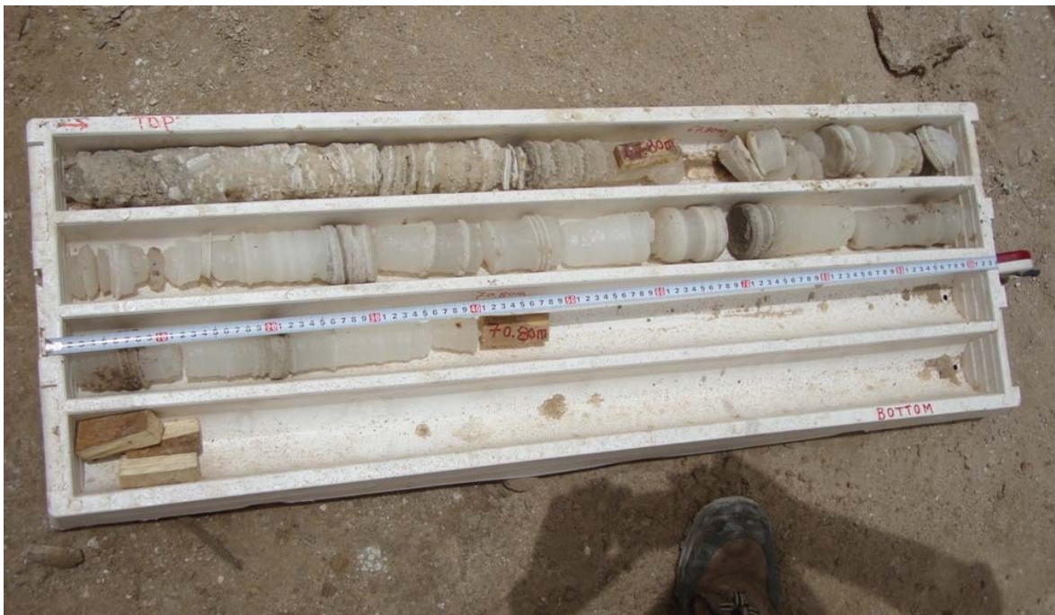
Figure 1 – Potash HQ core from COL-001 65.60m – 71.50m; note the dissolution of the core containing potash (core diameter is reduced), due to disruption to the equilibrium of the drilling mud composition.
