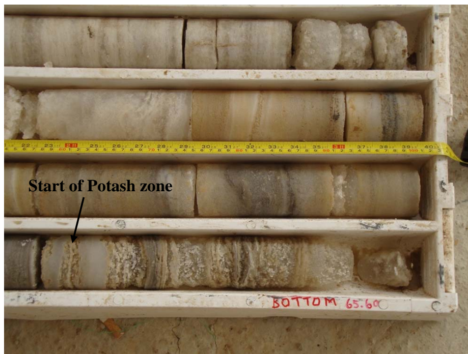
Figure 2 – Potash HQ core from COL-001 showing the start of the potash rich zone at ~65.00 m. Note the core recovery in the rock salt directly above the potash zone is very good and once into the zone it is reduced due to dissolution.
