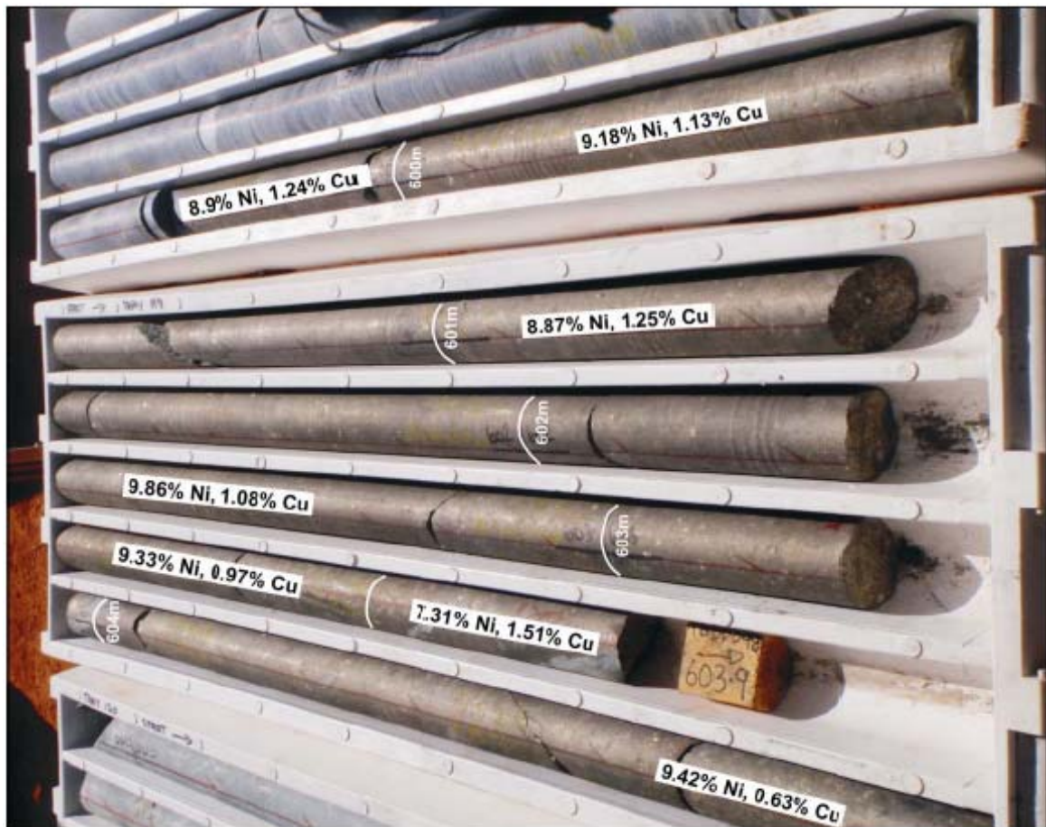
Figure 4 – JV Rosie Prospect - TBDD098 Massive Sulphide Intercept - 5.20m @ 9.13% Ni, 1.09% Cu, 0.21% Co and 7.09g/t PGEs (PGEs include 2.22g/t Pt, 1.74g/t Pd, 0.82g/t Rh, 1.79g/t Ru)
