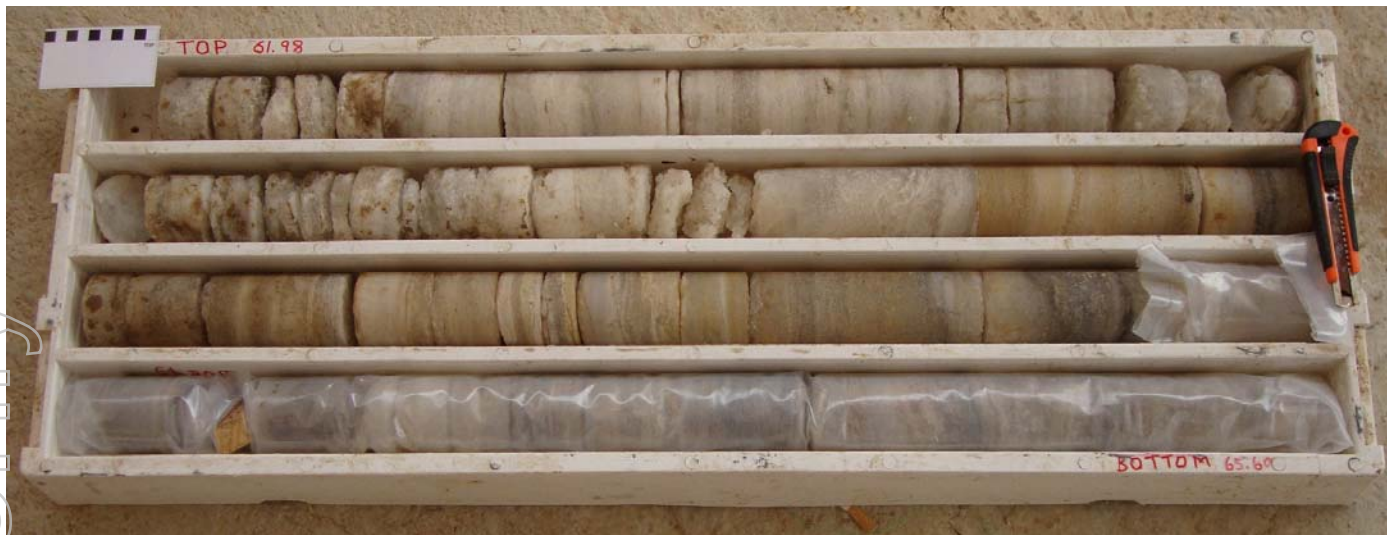
Figure 11 – COL-001 drill core showing rock salt and sylvite mineralisation from 61.98m – 65.20m.
