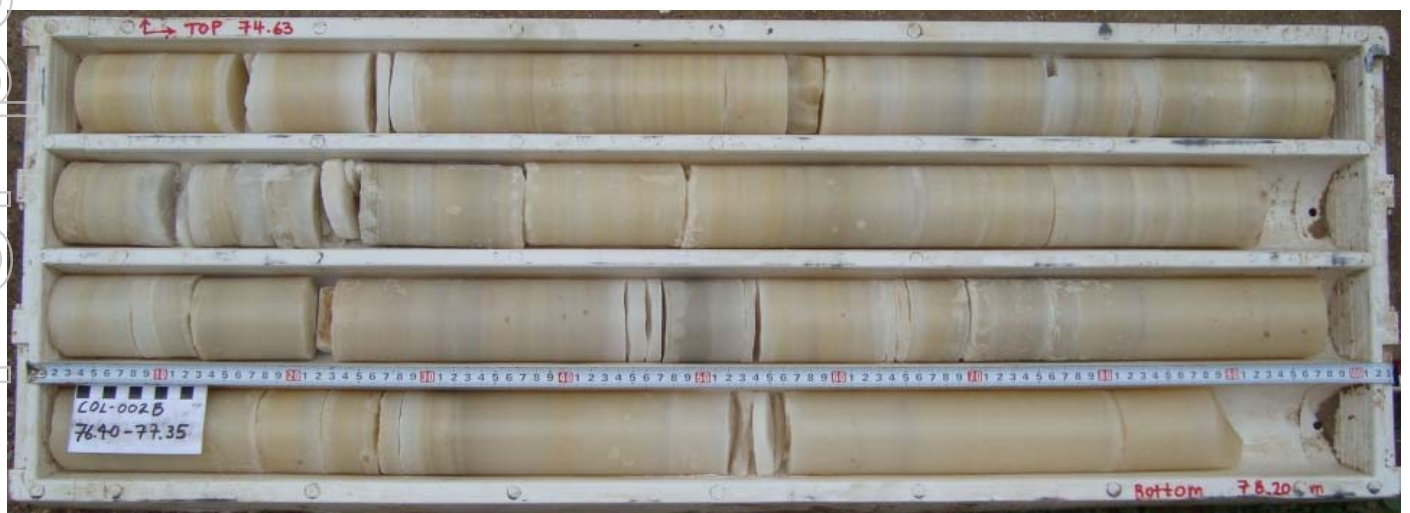
Figure 15 – COL-002B drill core showing kainite mineralisation zone from 74.63 – 78.20m.
