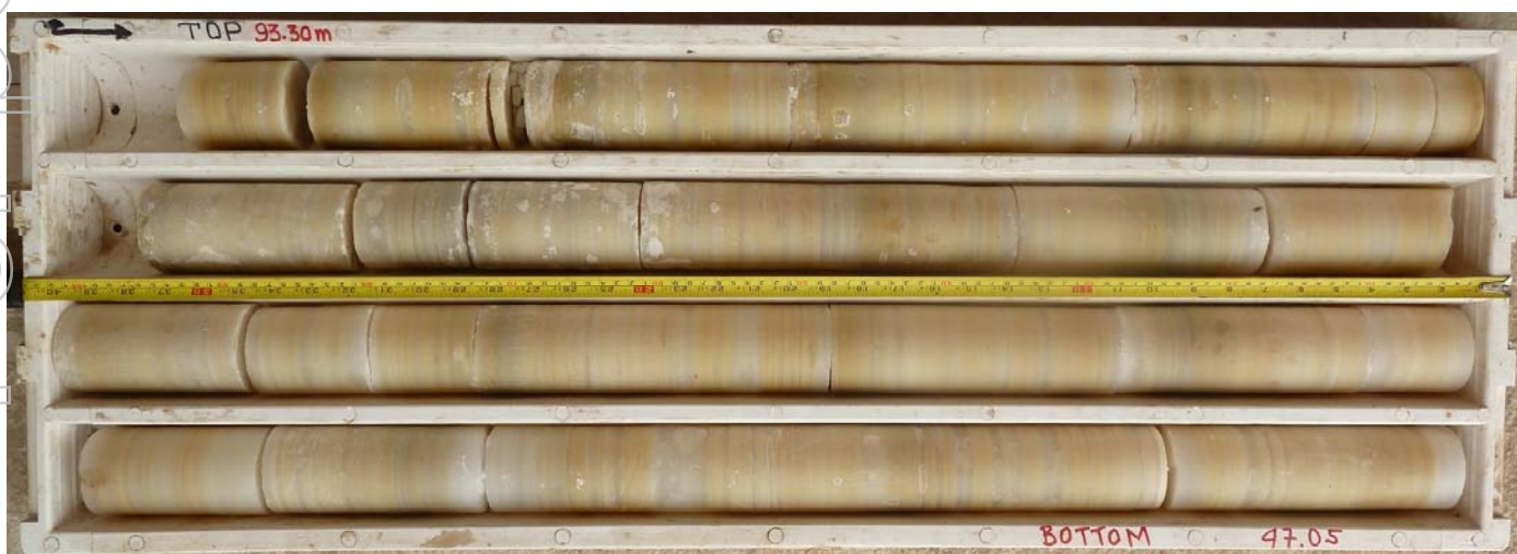
Figure 13 – COL-001 drill core showing kainite mineralisation from 93.30m – 97.05m.
