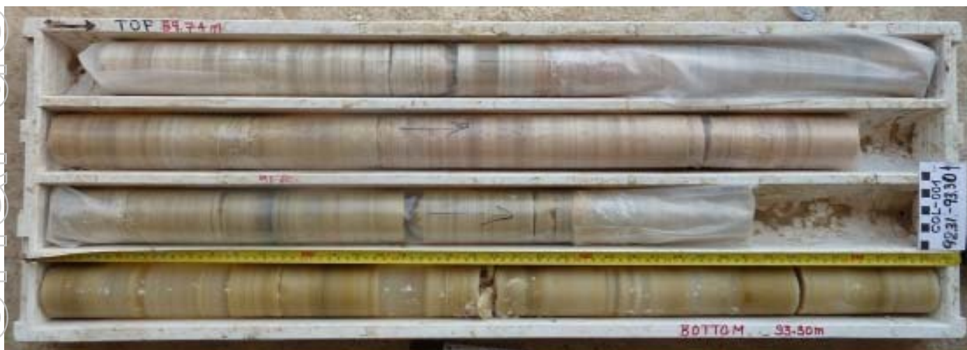
Figure 12 – COL-001 drill core showing base of strong carnallite mineralisation zone from 89.74 – 93.20m. Carnallite cores are heat sealed in plastic to prevent the core from dissolving in air.
