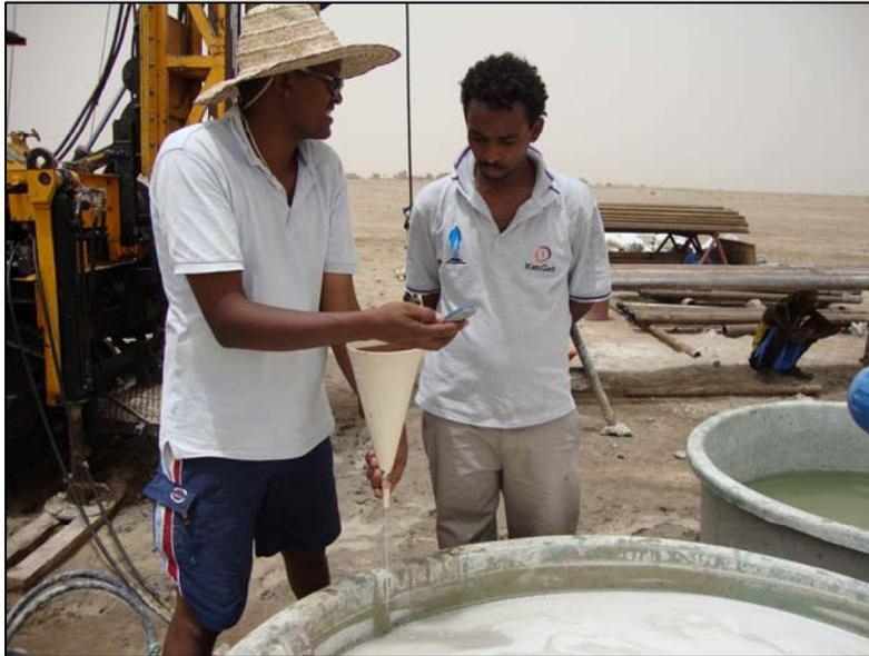
Above; Viscosity testing of diamond drilling mud for good recovery of the potash zones.
