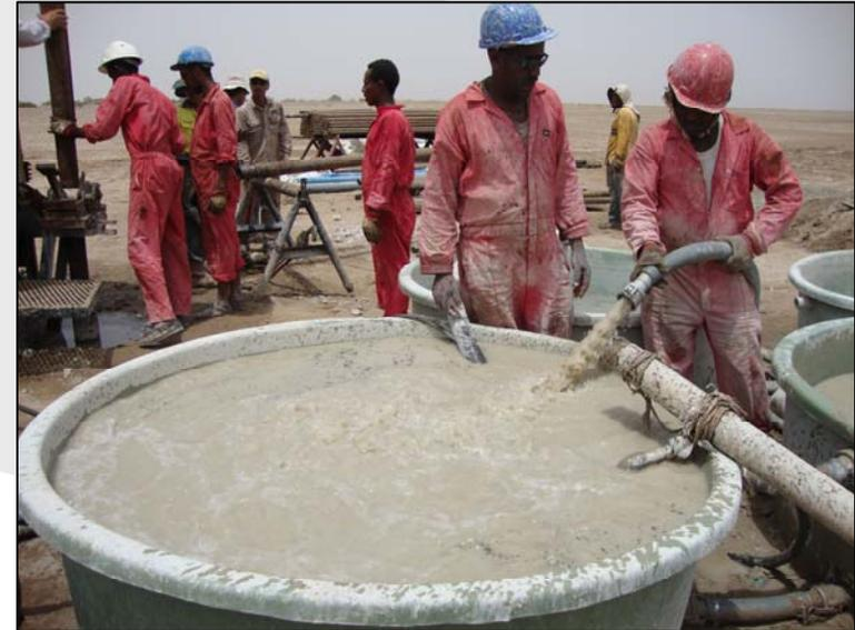
Above; South Boulder crew checking the important drilling mud.
