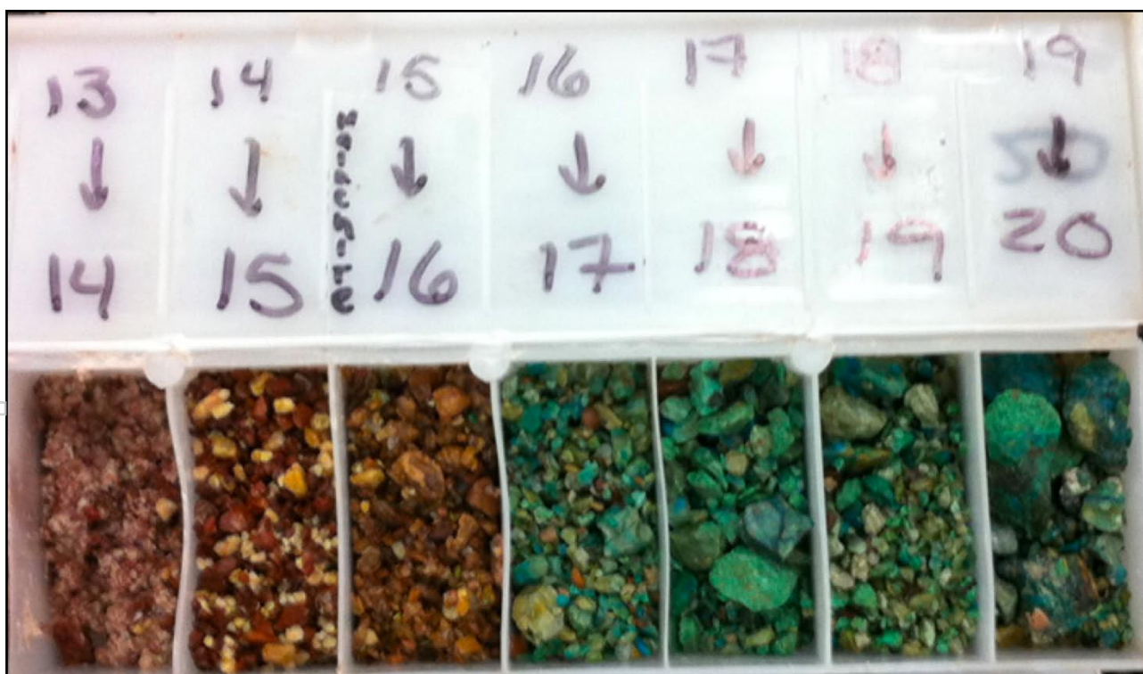
Figure 6. RC Drilling chips for 10BBC01 showing strong copper oxide mineralization 16-20m downhole.
