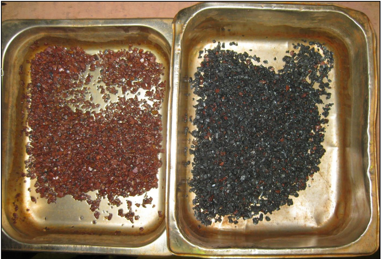
Figure 4. Composite 208-2, DMS Tail on left, DMS Concentrate on right.
