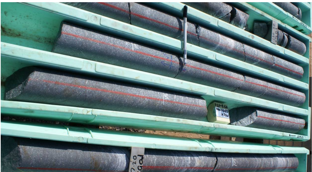
Figure 4. BUDD043 High grade coarse grained magnetite and hematite
