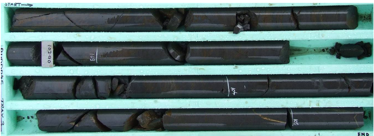
Figure 3. BUDD045 high grade magnetite silica BIF
