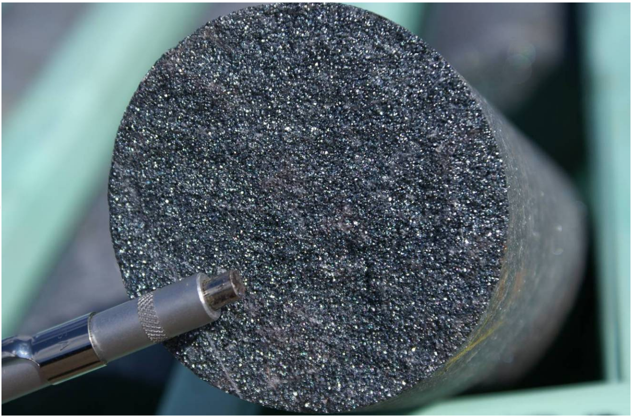
Figure 5. BUDD043 High grade coarse grained magnetite.
