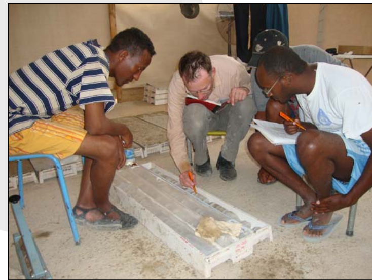
Logging potash drill core at Colluli.
