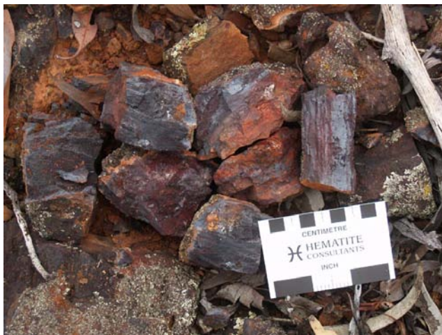
Figure 2. Surface Iron Enrichment in the form of Martite Goethite mineralisation
