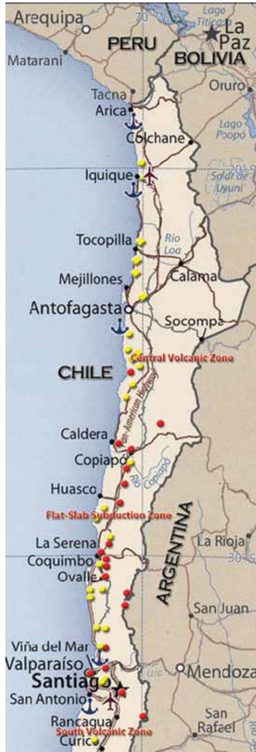
Figure 6. Copper-, silver-, gold-bearing veins, skarn deposits (Yellow = Cu-, Ag-, Au-,bearing veins; Red = skarn deposits)
