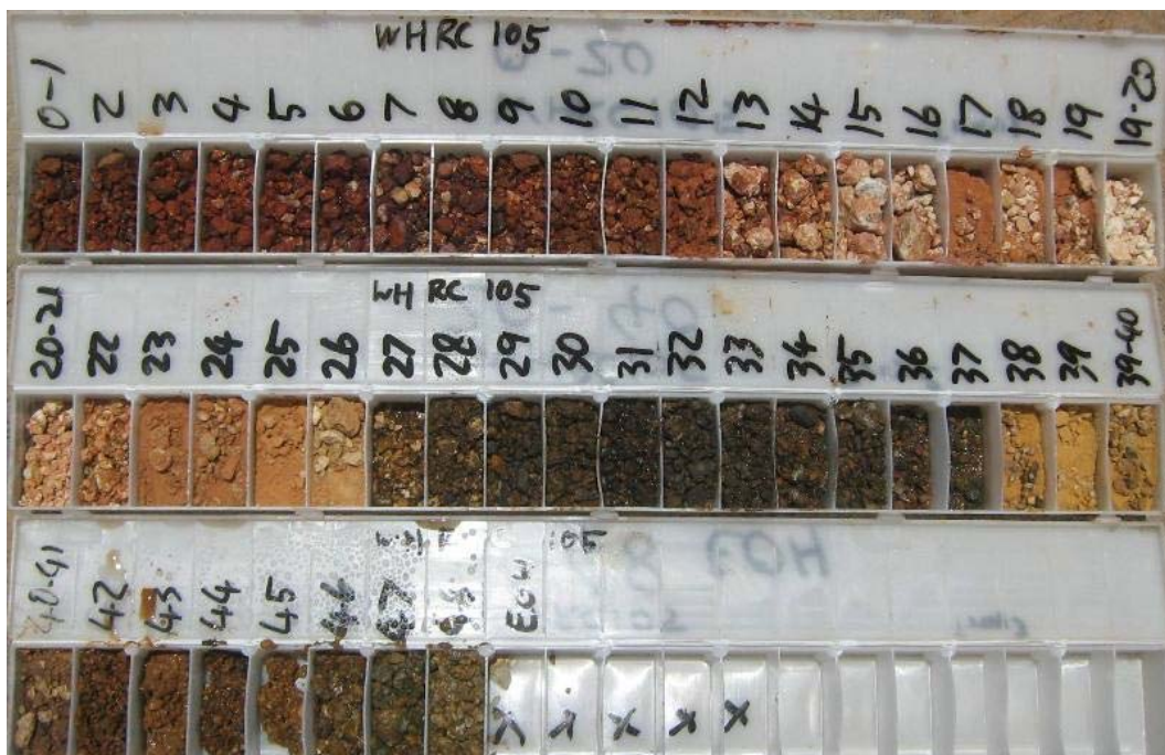
Photograph of Sieved Drill Cuttings from WHRC105
