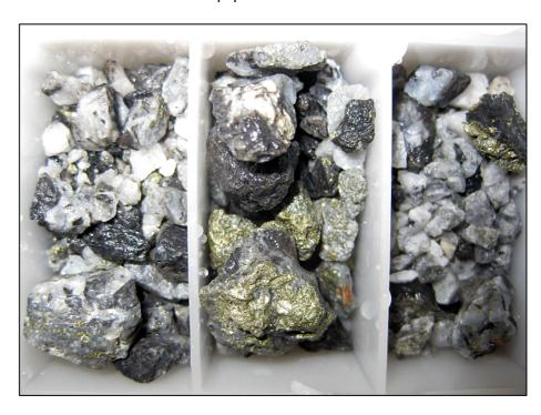
In addition to the copper minerals identified in hand specimen, other sulphide minerals can be seen in smaller concentrations in the drill spoil which suggests that the intersection may contain other commercially significant metals in addition to copper.
