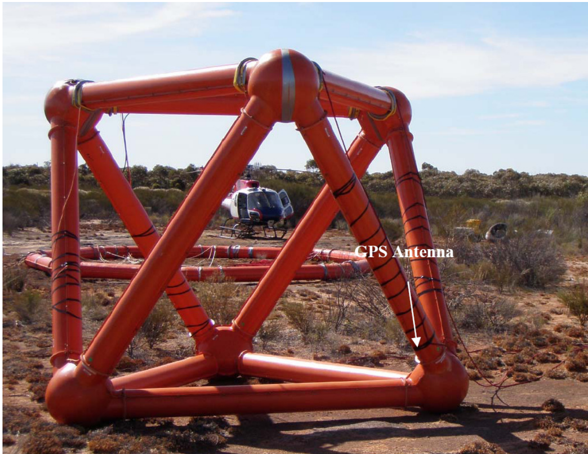
Figure 3 – ZTEM base station receiver coils
