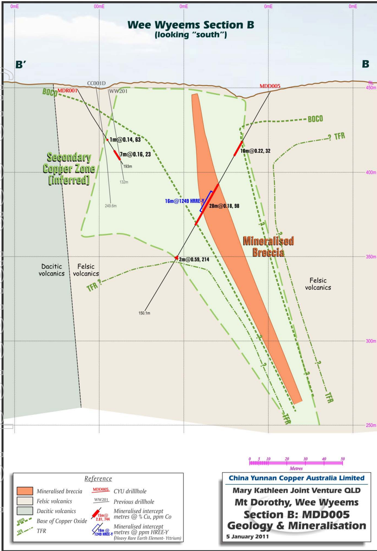
Figure 2. MDD005 section which confirmed NE trend of the mineralised breccia. TFR = Top of non weathered rock.
