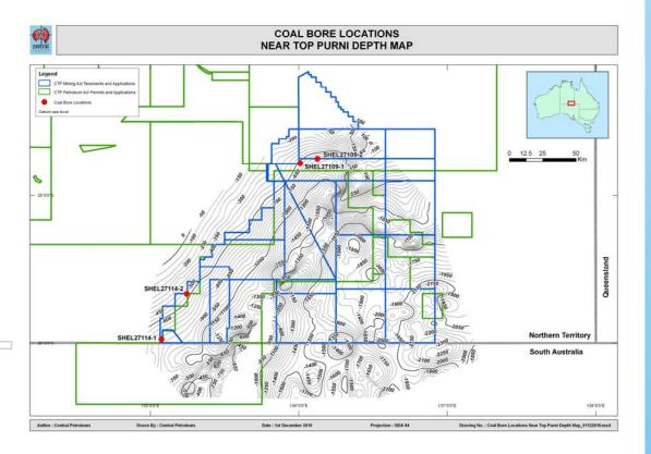
The first hole in the programme SHEL27109-2 was drilled to a depth of 1,209m MD prior to Christmas 2010 when the drilling contractor stood down for the Christmas/New Year break. The hole intersected approximately 33m of nett coal seams greater than 1m in thickness. It is possible that the programme may be redefined to include some drilling in anticipated shallower coal within three new mineral tenements EL's 28095, 28096 and 28097, the grant of which have been accepted by Central.
