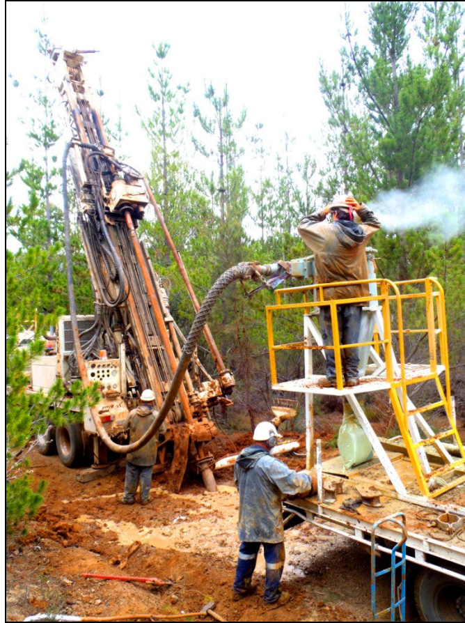
Figure 1 – Reverse Circulation drill rig at the Barnes Hill Project, Tasmania.
