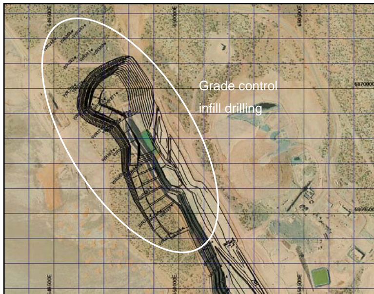
Start-up pit design (cutback of historic pit) with grade control drilling
