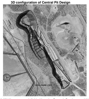
The planned pit length is 3.67 kilometers and divided into the Central, Southern and Northern areas. The Southern and Northern cutback extension of the existing pit will be mined to a vertical depth of 80 meters and the Central area has a maximum pit vertical depth of 155 meters. An average blend of 10% oxide, 25% transitional and 65% fresh ore is expected to be achieved over the life of the operation.
