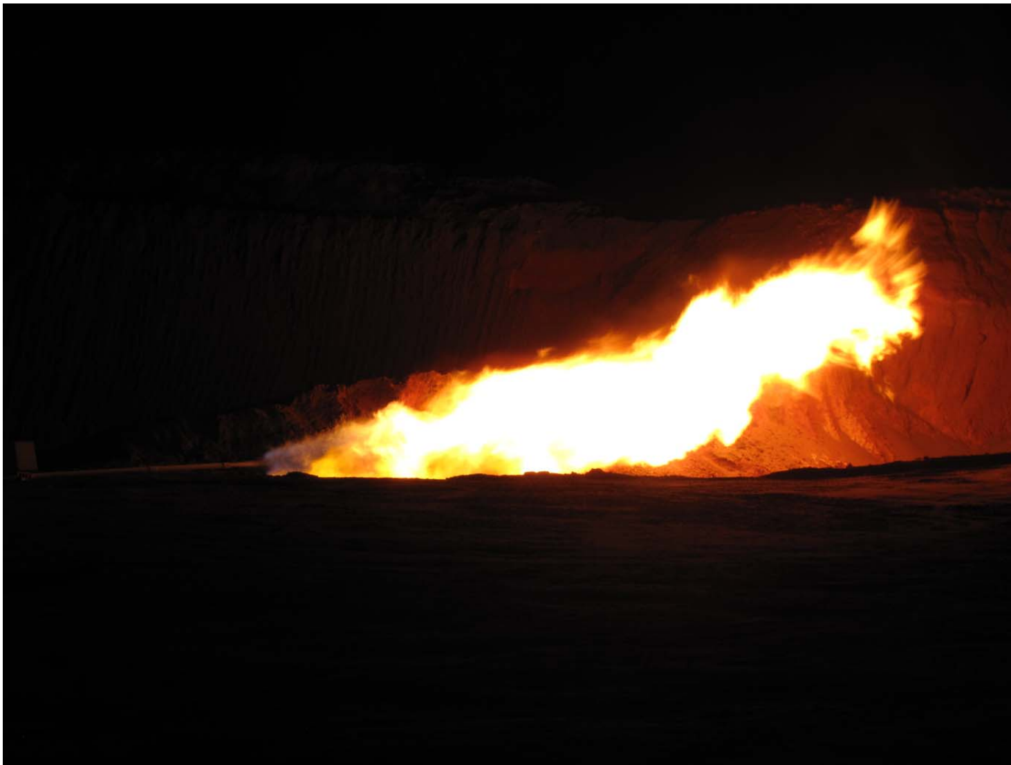
Red Gully-1 FARO 11.748 MMCFGD and 88 BCPD in enlarged Flare Pit
