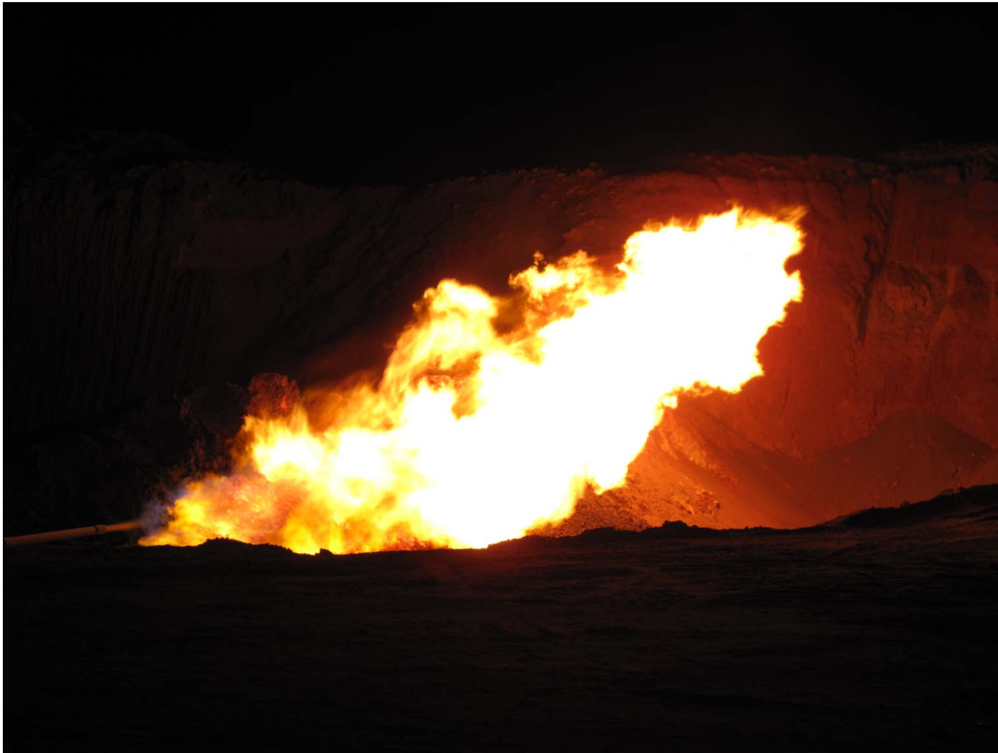
Red Gully-1 Flaring gas and Condensate on "cleaning up" after perforating
