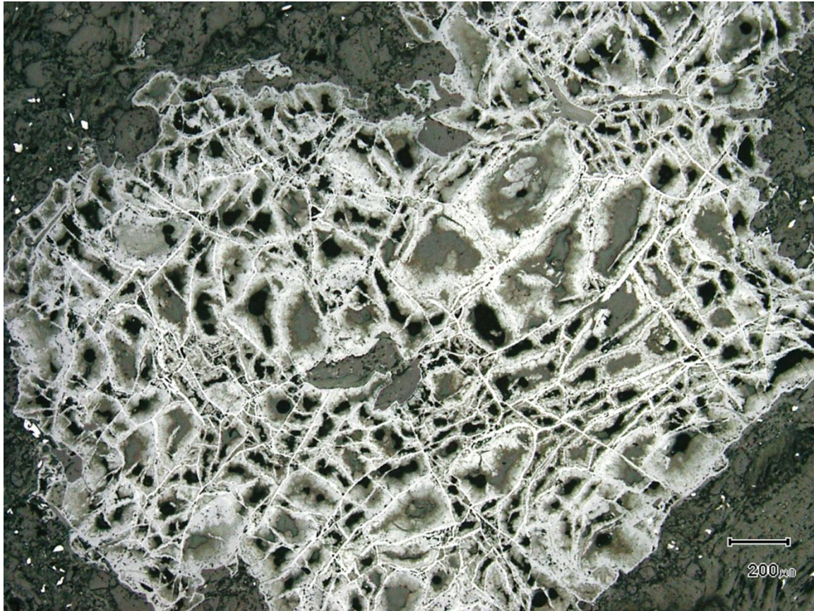
Figure 4. Polished section (PS), (x50). Gossanous/goethite box-work with a fine trellis texture interpreted to represent original chalcopyrite now completely oxidised and leached.
