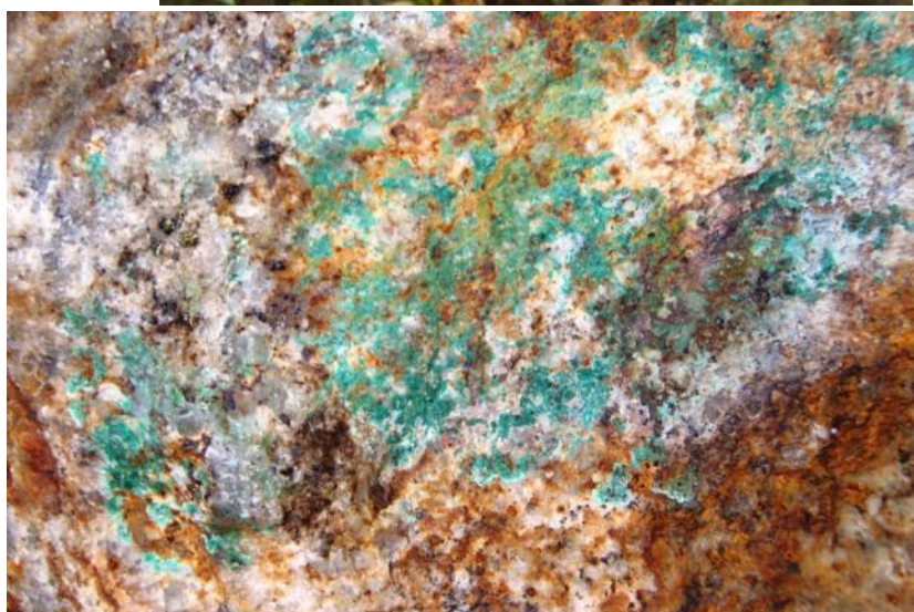
Figure 7. Secondary copper mineralisation on the fracture face of a porphyritic rock from Andewa at approx. real (100%) scale.
