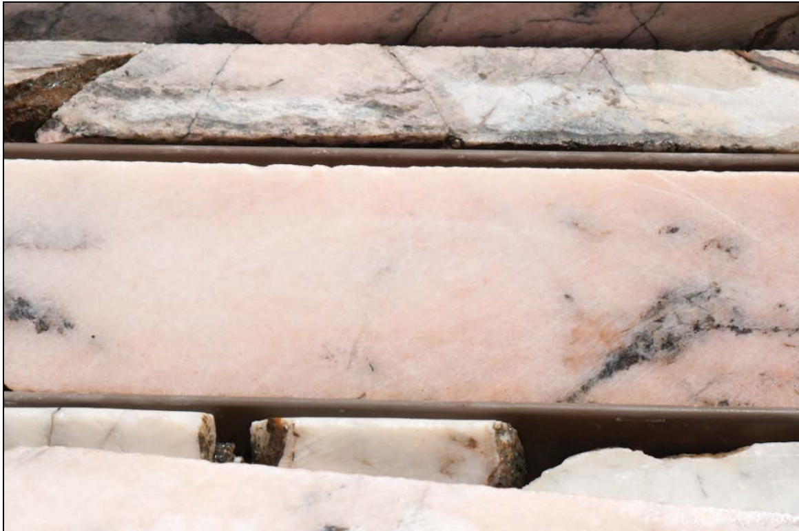
Figure 4-13: Drillcore from Cummins Range in the carbonate rich fresh zone CDD001 at ~152.5 m showing the massive pink coloured carbonatite with some mica rich zones.
