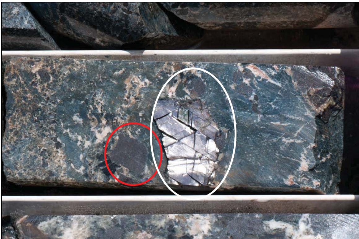
Figure 4-14: Drillcore from Cummins Range in the pyroxenite rich fresh zone showing coarse-grained magnetite CDD001 at ~97.5 m showing the coarse-grained magnetite (red circle) and mica (white circle) within a poorly foliated pyroxenite.
