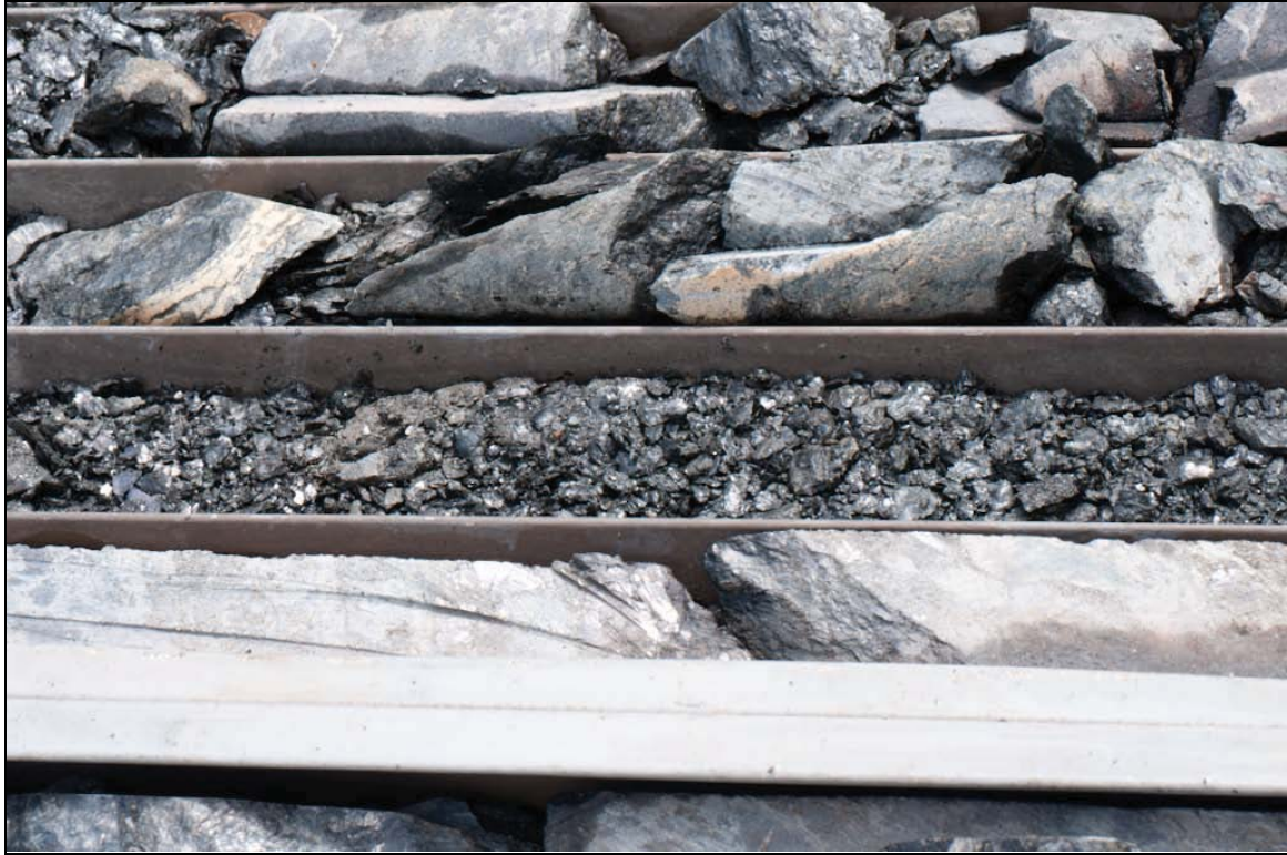
Figure 4-15: Drillcore from Cummins Range in the pyroxenite rich fresh zone CDD001 at ~187 m showing the highly foliated pyroxenite.
