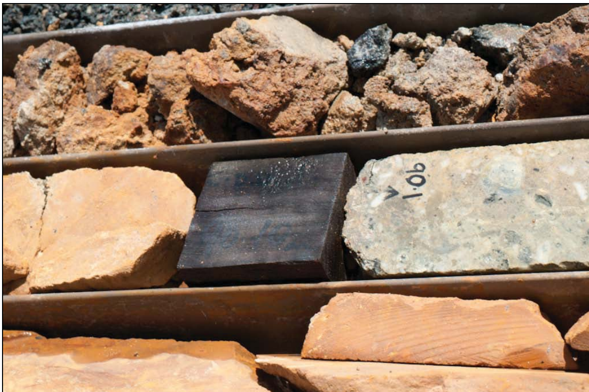
Figure 4-16: Drillcore from Cummins Range showing the contact between fresh and weathered CDD001 at ~90.1 m.
