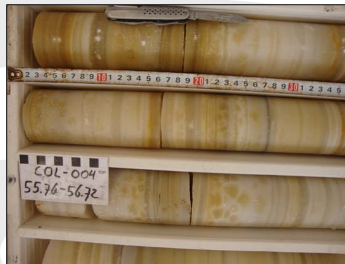
COL-004 drill core showing high grade carnallite and kainitite mineralisation.
