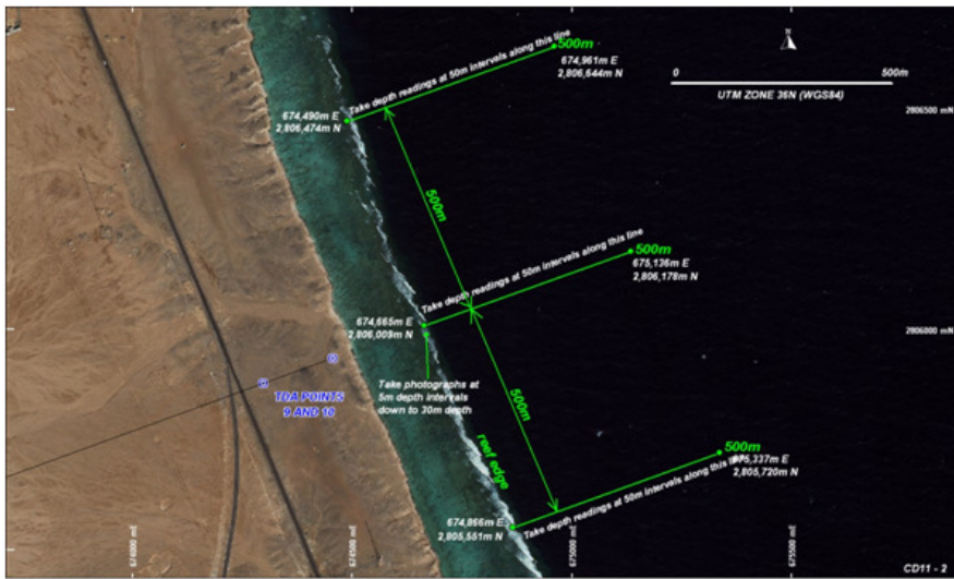
Diagram 4: Location of Bathymetric Survey Lines
