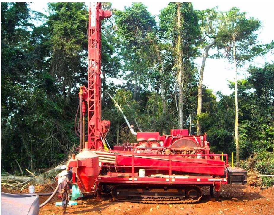
FIGURE 4: RC DRILLING AT THE NABEBA DEPOSIT DURING MARCH QUARTER
