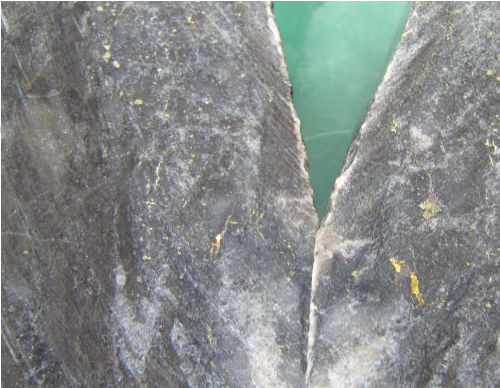
Figure 4: Visible Gold in Diamond Hole 11GYD0005. Yellow specks are Coarse and Fine Gold, Silvery Specks and Veinlets are Sulphides and Dark/Black Veinlets and Blobs are Molybdenite.
