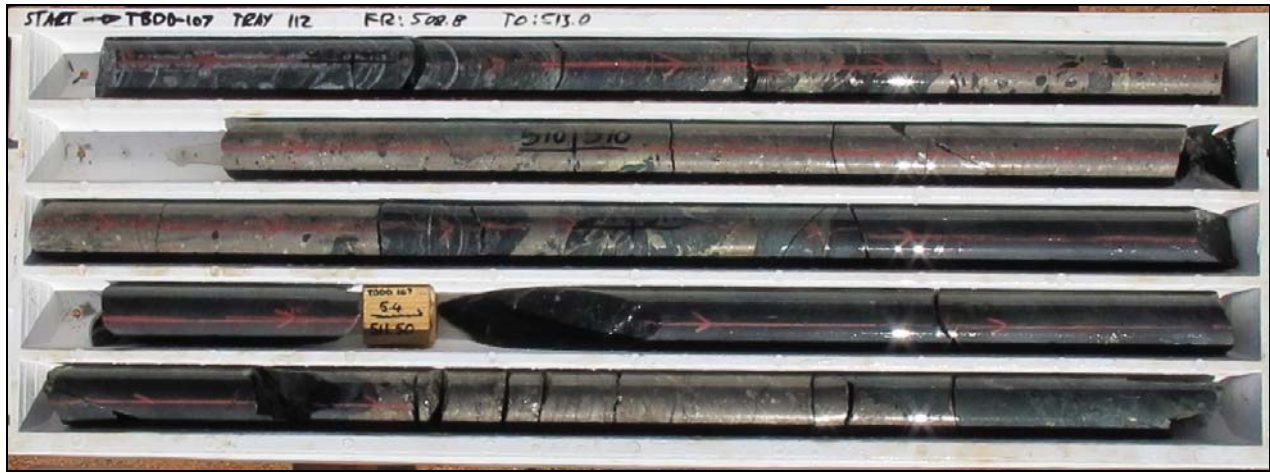
Figure 5 - Rosie Prospect hole TBDD107 showing massive sulphides.
