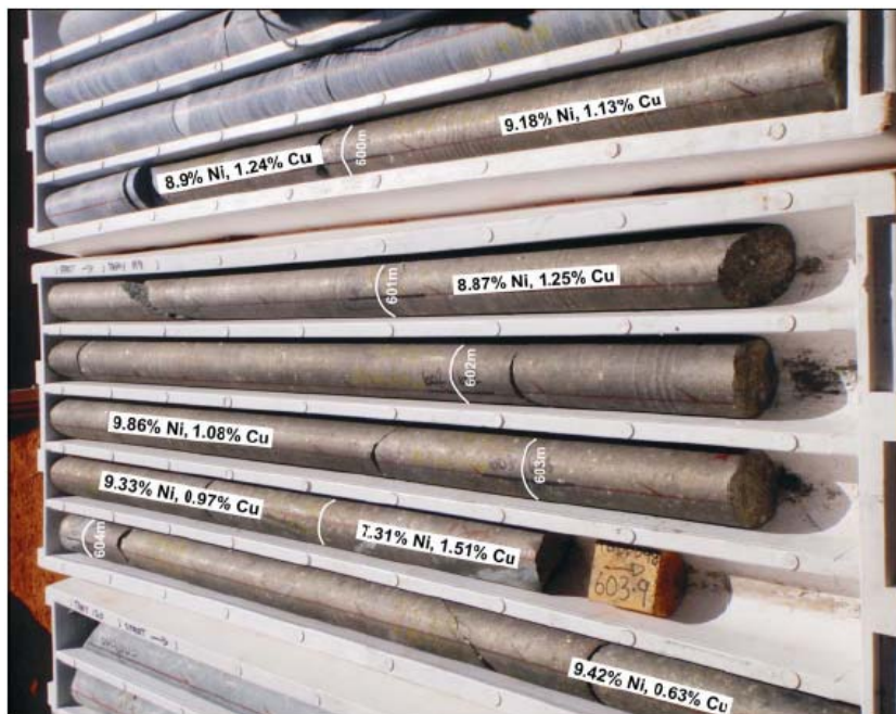
Figure 4 – Duketon Nickel JV Rosie Prospect - TBDD098 Massive sulphide intercept - 5.20m @ 9.13% Ni, 1.09% Cu, 0.21% Co and 7.09g/t PGEs (PGEs include 2.22g/t Pt, 1.74g/t Pd, 0.82g/t Rh, 1.79g/t Ru
