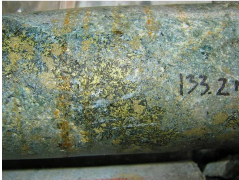
Figure 7: TTDD011 133.2m Quartz-sericite-tourmaline-pyrite-chalcopyrite alteration of quartz diorite (132-134m: 0.7 g/t Au, 2700ppm Cu)
