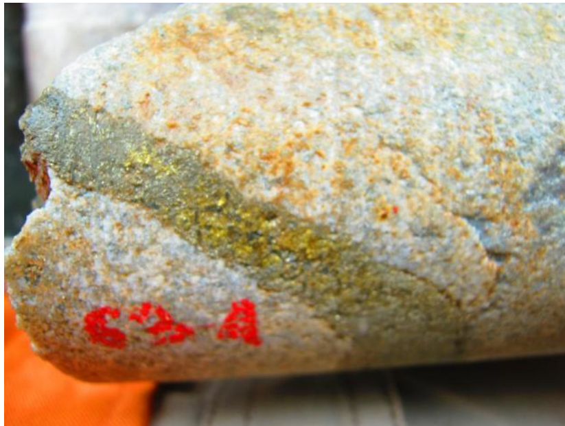
Figure 8: TTDD011 63.4m Quartz-pyrite-chalcopyrite veining in quartz-sericite-pyrite altered quartz diorite (62-64m: 3.04 g/t Au, 1310 ppm Cu)
