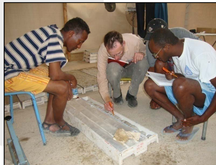
Logging potash drill core at The Colluli Potash Project, Eritrea.
