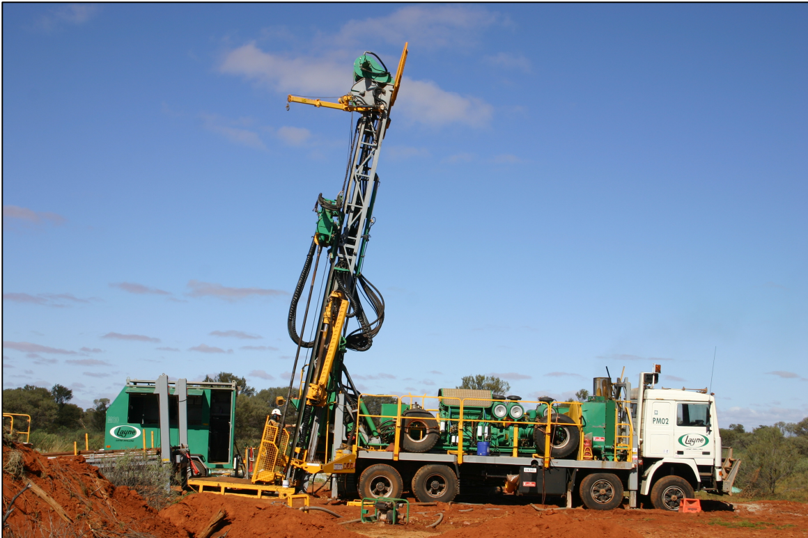
Figure 3: Diamond core drill rig.
