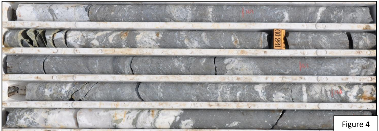
Figure 4. Close-up central part of main base metal massive sulphide intersection.
