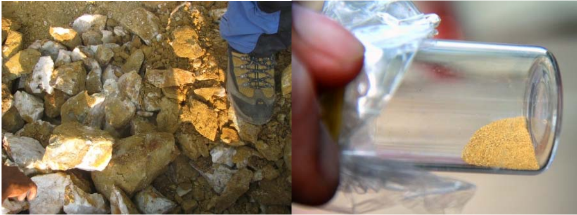
Fig. 5: Kratie North, Target #2 - Gold-bearing Vein material; Example of gold recovered from Veins
