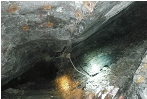
855 stope drive showing the neat extraction of the gold ore and the favorably strong hanging wall. The Level drive is 3m high and the stope about 1m average height.
