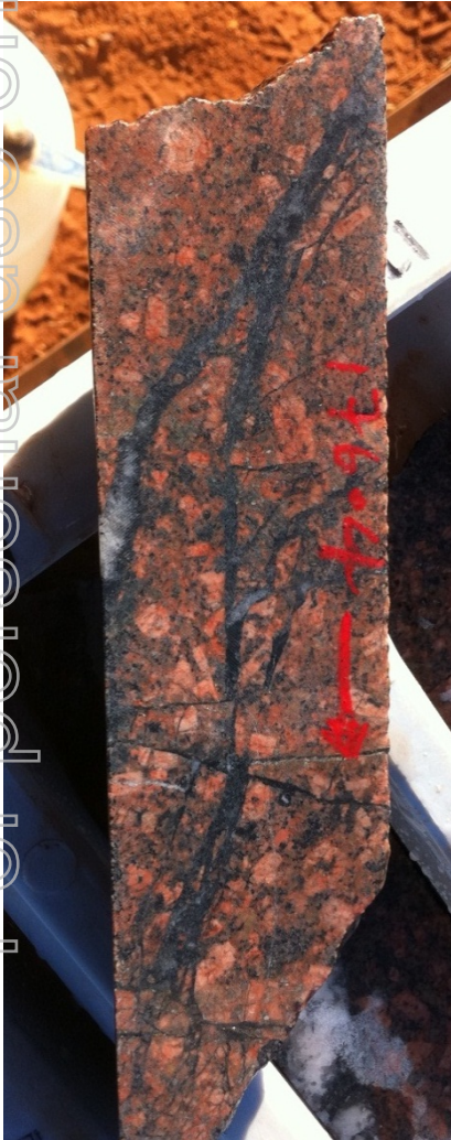
Chlorite / Biotite / Qtz fractures / stock-working in porphyry – typical grade 0.2 to 1.5g/t Au over wide widths.
