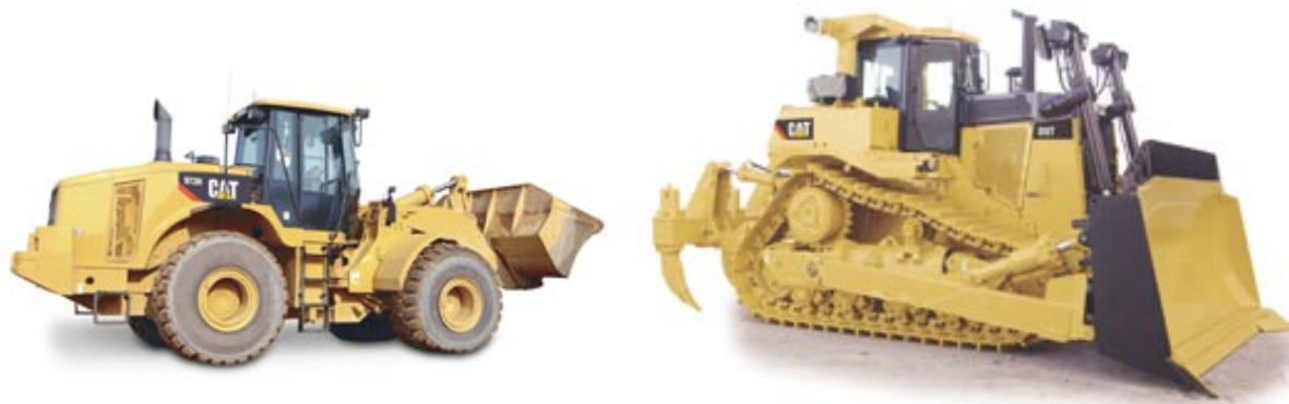
Figure 1 – 972H Wheel Loader (left) and D10 Dozer (right) for Mining at Barnes Hill
