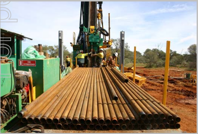
Diamond Core drilling
